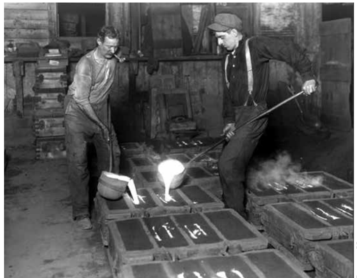
Pouring iron at Rathbone & Sard foundry, Albany, N.Y., c. 1911.
